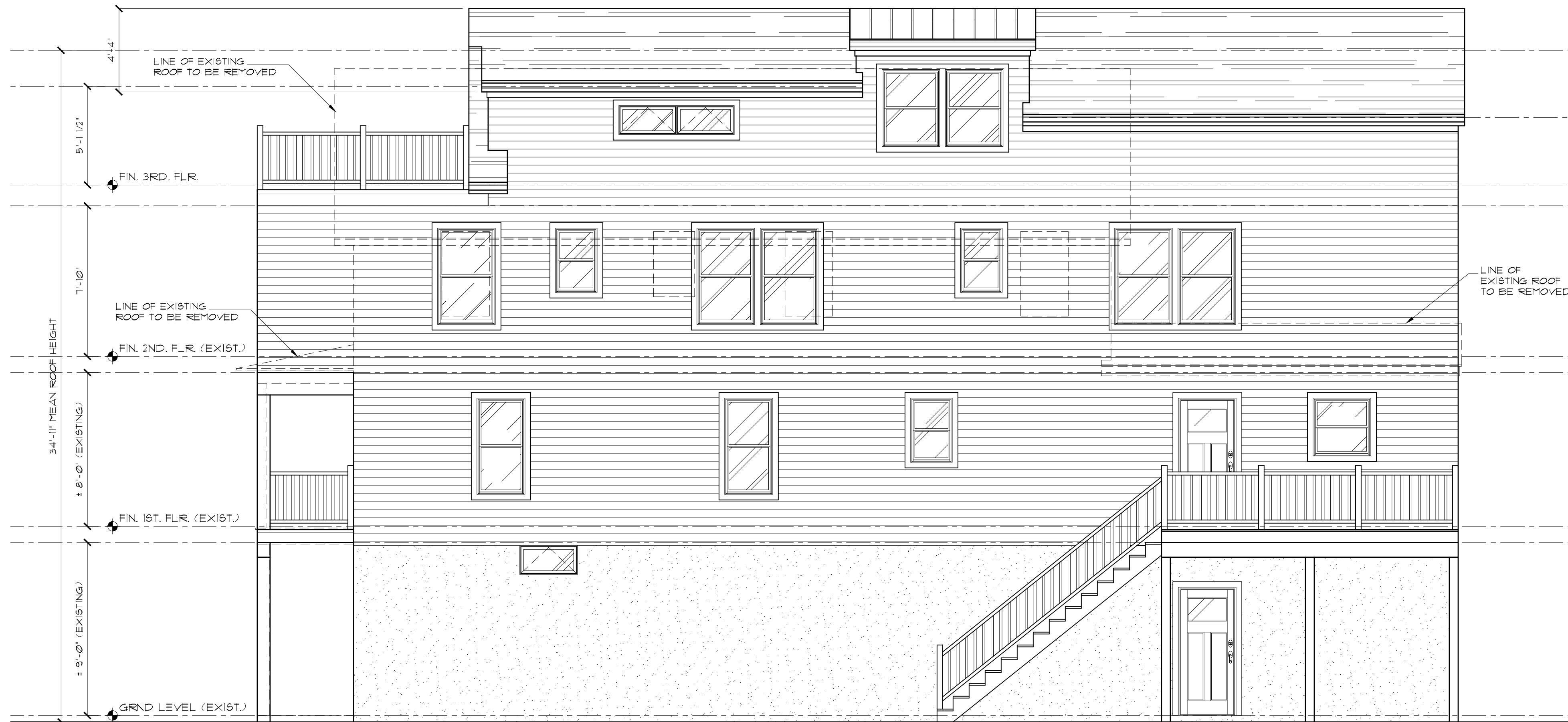
RIGHT SIDE ELEVATION SCALE: 1/4" = 1'-0"
